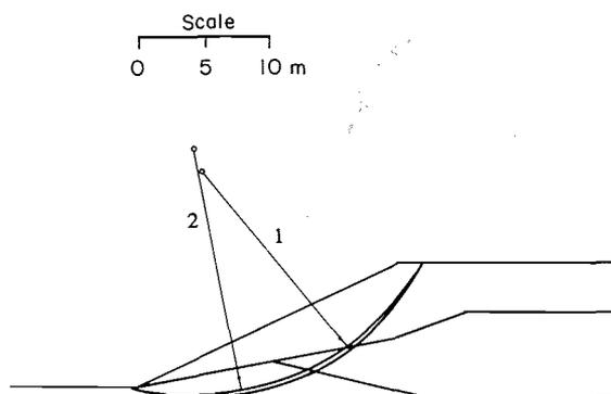
FIG. 5. Comparisons between the results obtained by the Bishop's simplified method and the simplified method 1 for the example shown in Fig. 1a (horizontal seismic force coefficient = 0.15g). The critical slip surfaces: 1, obtained by the Bishop's simplified method,  $F_m = 1.006$ ; 2, obtained by the simplified method 1,  $F_m = 0.967$ .
