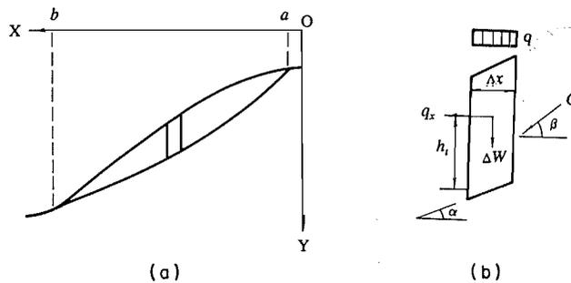
FIG. A1. The limiting equilibrium of a slope analyzed by the method of slices. (a) Stability analysis along a potential slip surface. (b) Forces applying on a slice.
