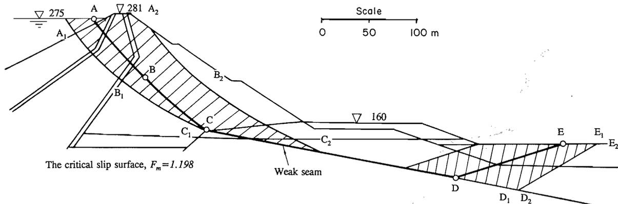
FIG. 7. Stability analysis of the downstream slope for the Xiaolangdi rock-fill dam.
