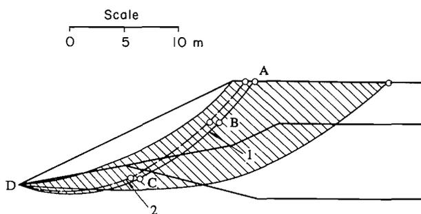
FIG. 4. Search for the minimum factor of safety for the problem shown in Fig. 1a. Slip surfaces: 1, the initial estimate, determined by the random search,  $F_0 = 1.384$ ; 2, the critical, obtained by the Simplex method,  $F_m = 1.373$ .
