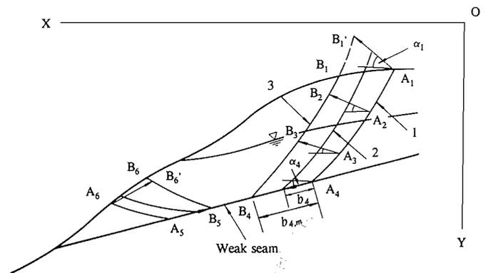
FIG. 2. Slip surfaces of generalized shape. 1,  $Z^0$ , the initial estimate; 2,  $Z$ , the slip surface during the process of optimization; 3,  $Z^m$ , the critical slip surface.
