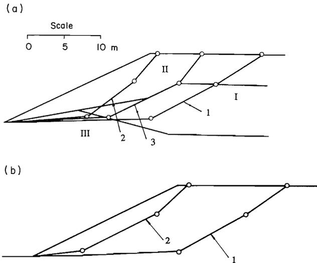
FIG. 1. An example displaying the success and failure of the searches for the minimum factor of safety. (a) A layered slope. Slip surfaces: 1, the initial estimate,  $F_0 = 1.951$ ; 2, the known critical slip surface,  $F_m = 1.484$ ; 3, the slip surface at which the calculation terminates,  $F = 1.511$ . (b) A uniform slope. Slip surfaces: 1, the initial estimate,  $F_0 = 1.576$ ; 2, the critical slip surface at which the calculation terminates,  $F_m = 1.006$ .
