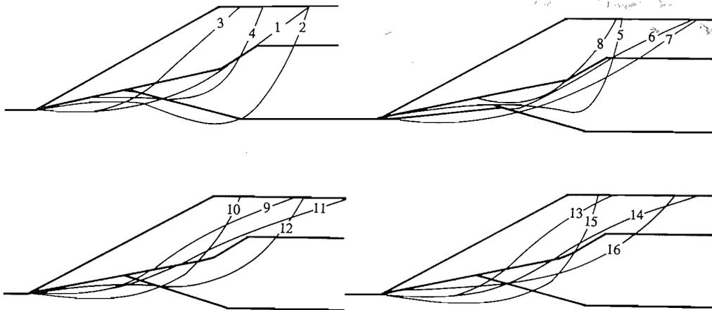
FIG. 6. The random slip surfaces generated in the search area shown in Fig. 5. Refer to Table 4 for factors of safety.
