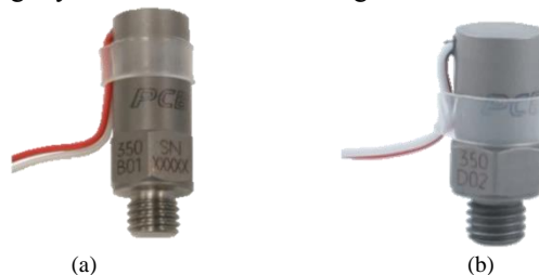
Figure 5 Accelerometers used in the test. (a) 350 B01; (b) 350 D02.
